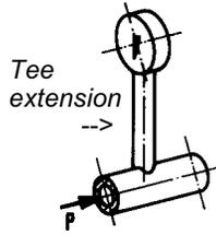
With a gaseous pressure medium, the extension should have a drain plug at its lowest point, while a line with a liquid medium should have an air bleeding valve at its highest point. A filter or separator should be used when the pressure medium contains suspended matter.
